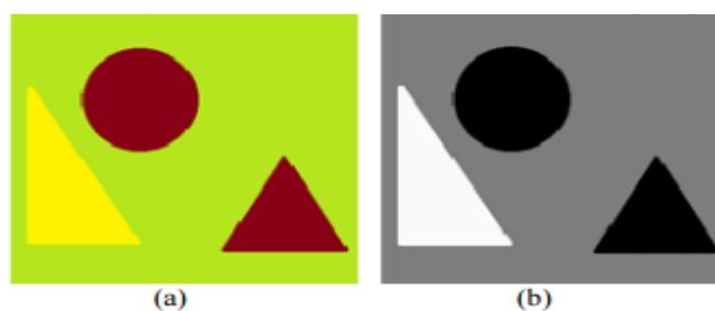
Figure 1.3: Example segmented image (a) an image of three objects and (b) the result of image segmentation.
